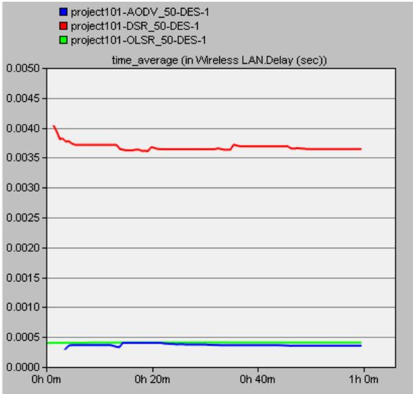
Figure 3.5 : End-to-end delay –50 sources at 30m/s
