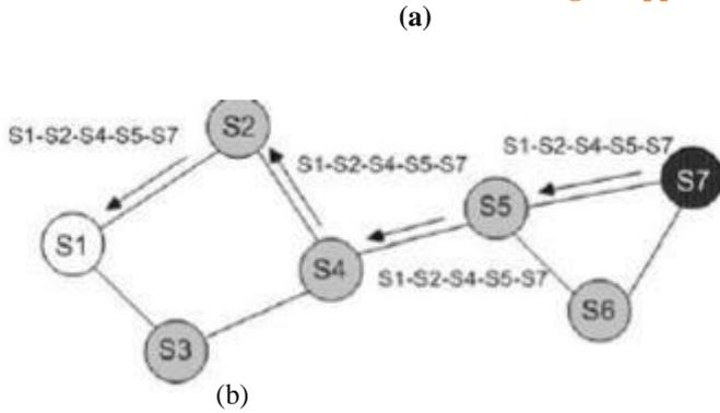
Fig. 1.3 (a) Route Discovery (b) Using route record to send the route reply
