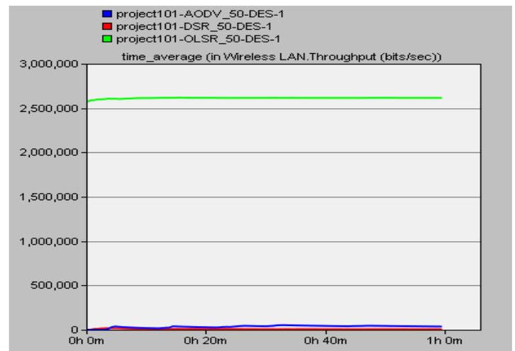
Figure 3.9: Throughput –50 sources at 30m/s
