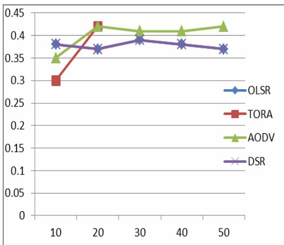
Figure 3.6: Packet delivery ratios at 10 m/s
