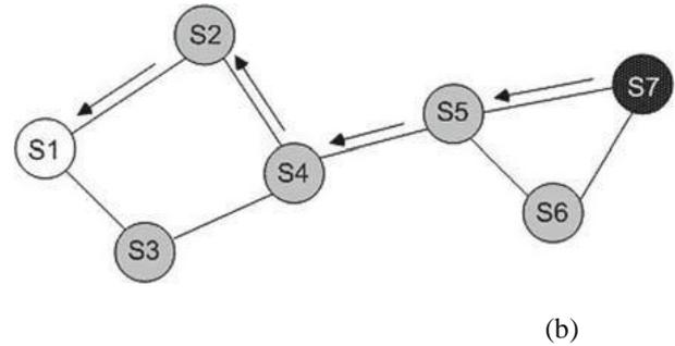
Figure 1.2 AODV protocol (a) Source node broadcasting the route request packet. (b) Route reply is sent by the destination using the reverse path
