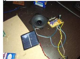
Fig 2.7 Audio receiver with solar panel
