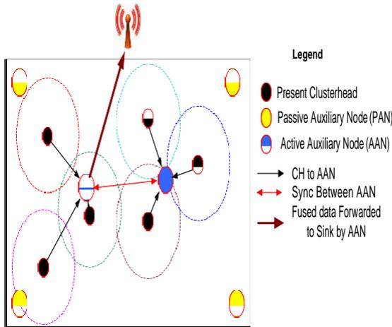
Fig.1 Proposed Communication Model
