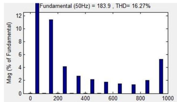
Fig.4. Output voltage frequency spectrum for Fig. 3
