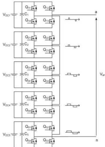
Fig. 1. Cascaded inverter: (a) topology and (b) output waveform
