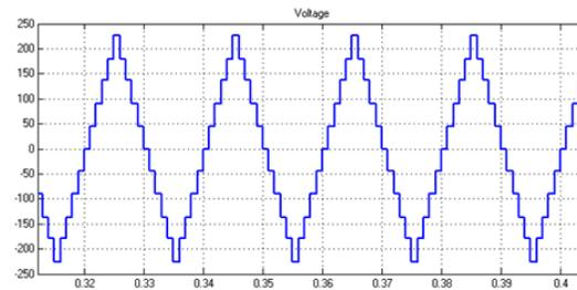
Fig.3. Multilevel inverter line output voltage waveform.
