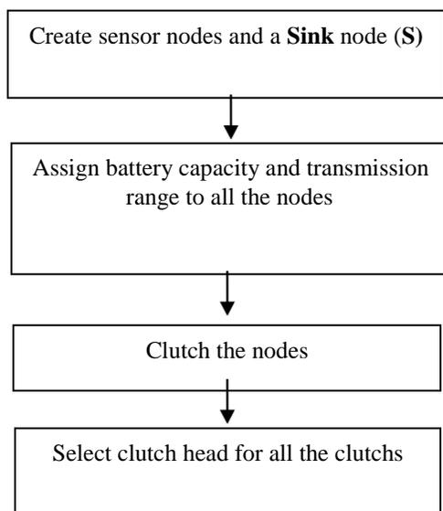
**Figure. 6. Clutch head selection K Means Clustering Algorithm**
