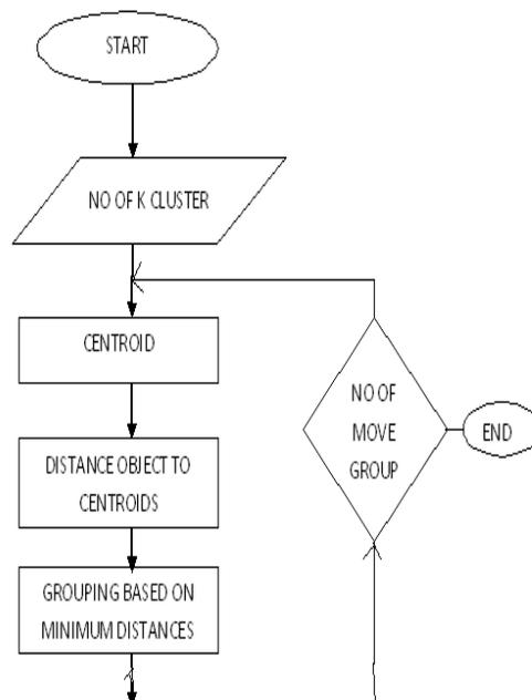
**Figure. 7. Flow diagram of k means algorithm**
