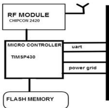
**Figure 4** Body sensor Node
