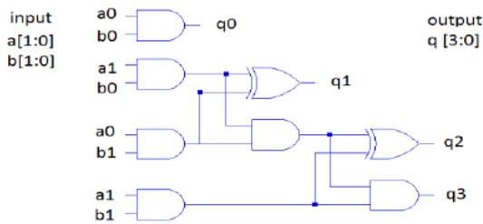
Fig.3: 2-bit Vedic multiplier using logic gates .
