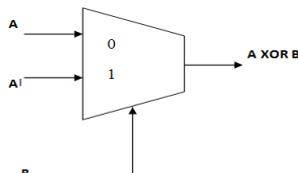
By using these multiplexers 2-bit vedic multiplier using multiplexers is designed by replacing AND, OR, and XOR gates by multiplexers is shown in Fig.5.
