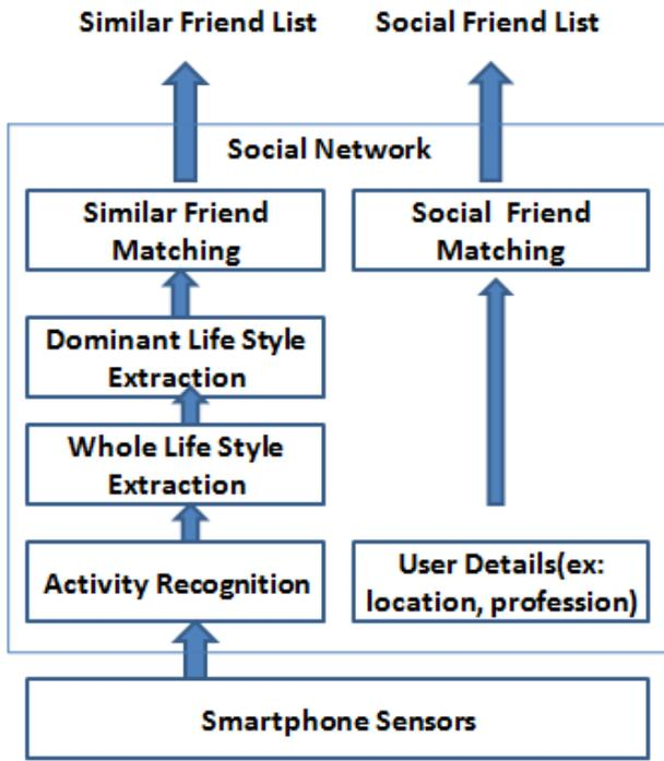
Fig. 1. System architecture of Friend Recommendation system.
