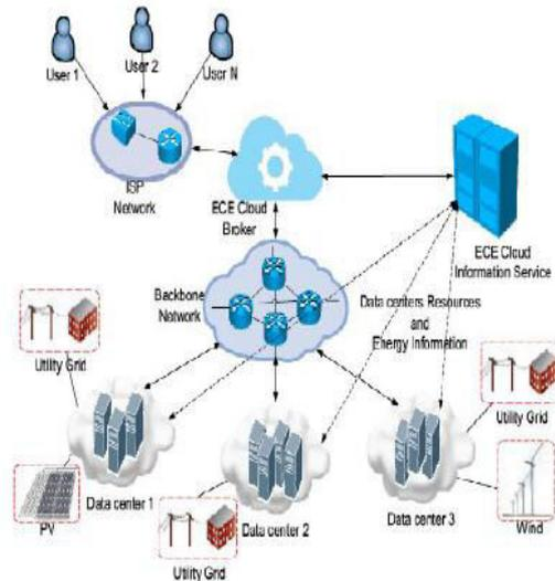
Figure. 5 Energy and Carbon-Efficient (ECE) Cloud Architecture[22]
