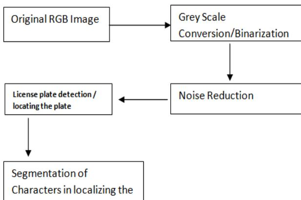
**Fig.2. Structure of ANPR system**
