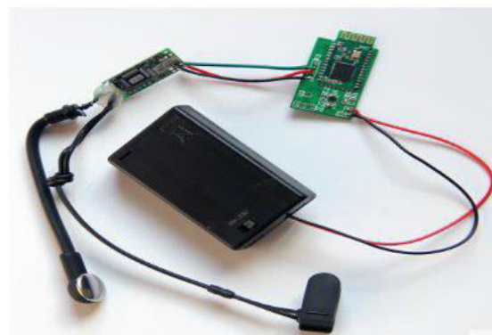
Figure 2: Brain sensor headset components
