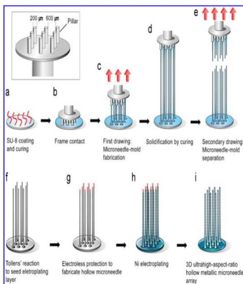
Fig. 1 demonstrate the sequential procedure and steps involved in the fabrication of the micro-needles employing the photo-patterning method of SU-8. (a) deposition of SU-8 by spin coating method; (b) frame pattern contact for drawing; (c) drawing of deposited SU-8 polymer layer; (d) curing through thermal cross linking of drawn SU-8; (e) secondary drawing to develop micro-needle pattern; (f) development of the seed layer using electroplating; (g) fortification of
