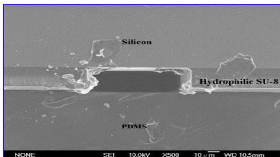
Fig. 3 SEM image shows the bonding location between Si and PDMS substrates. The inserted microchannel is of size 100 X 34 μm<sup>2</sup>[13].
