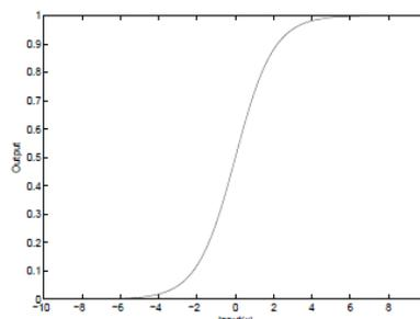
Fig. 2. Shape of a original sigmoid function
