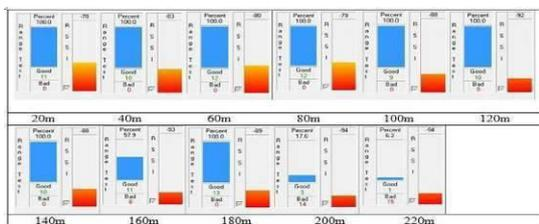
Fig 14: X-CTU screen for outdoor Measurement of RSSI value at transmit power level P4.
