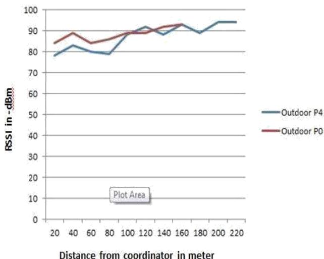
Fig 11: Measurement of RSSI value vs. distance at transmit power level P0 and P4.
