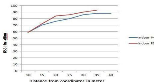
Fig 10: Measurement of RSSI value vs. distance at transmit power level P0 and P4.
