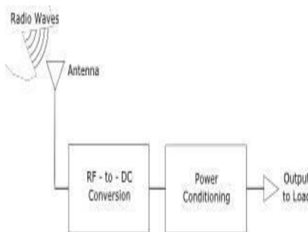
Fig. 2. RF Based Energy Harvesting Structure
