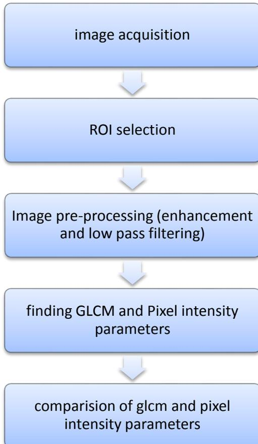
Fig (1) Block diagram
