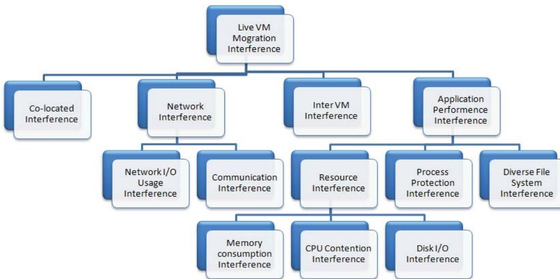
**Figure 3: Classification of Interference introduced due to the VM migration**
